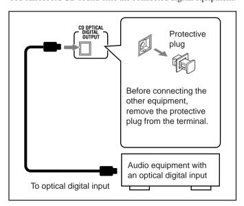
Connect an optical digital cord (not supplied) between the optical digital input terminal on the other equipment and the CD OPTICAL DIGITAL OUTPUT terminal.
