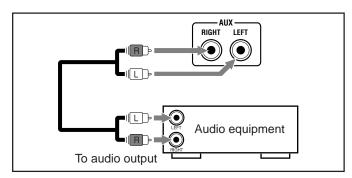
For playing the other equipment through this unit, connect between the audio output jacks on the other equipment and AUX jacks by using audio cords (not supplied).
